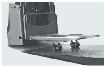
Best suited to ramps: initial lift helps the EXV drive up ramps with ease
