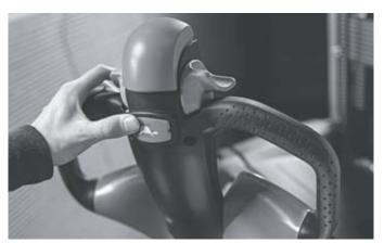
Precise in all situations: creep speed also makes it possible to manoeuvre in the most confined of spaces
