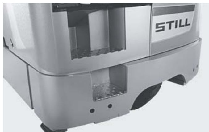
Safe entry thanks to additional step
