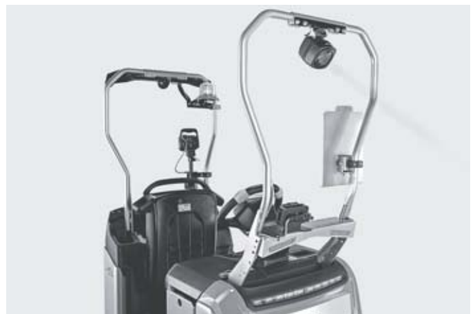
Excellent vehicle visibility thanks to optional Safety Light and Safety Light 4Plus for maximum driver safety
