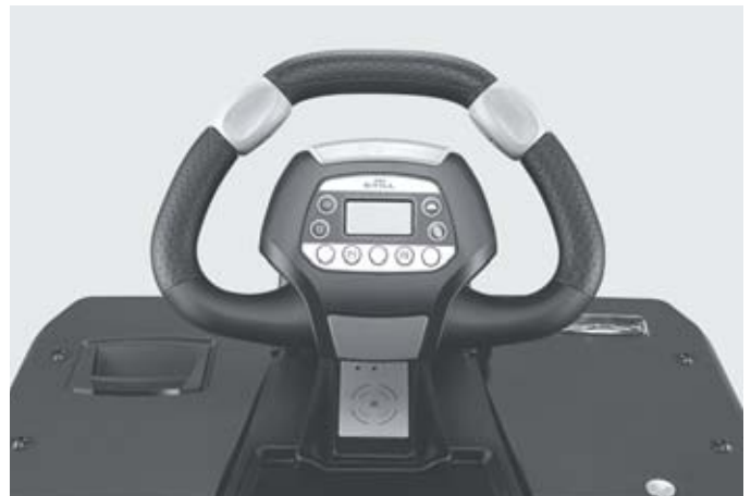
Unique STILL Easy Drive steering wheel for optimised driver control and operation of all functions without changing grip
