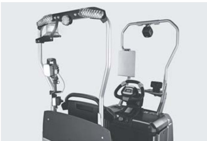
Optional accessory bar for versatile application options and many equipment options including flash lights and working lights
