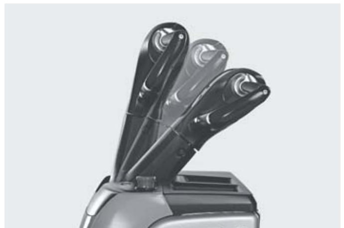
Height-adjustable steering for different drivers
