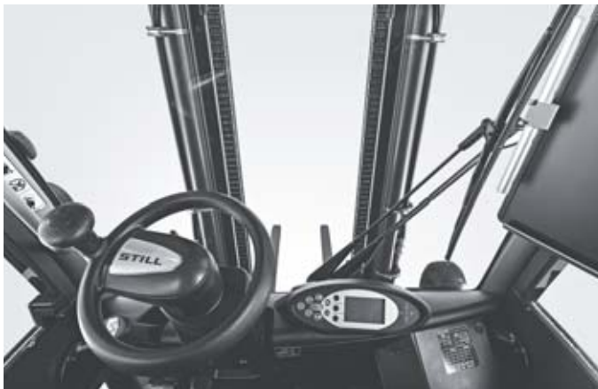
Excellent visibility to the front due to clear-view mast and low dash panel
