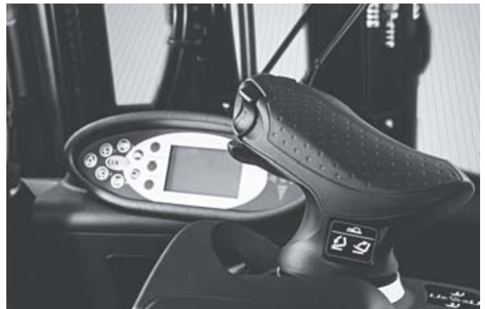
Convenient and precise hydraulic operation with the Joystick 4Plus
