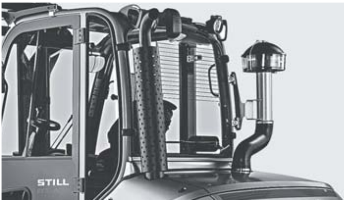
Cyclone air filter for clean engine intake air
